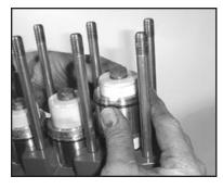
7. For LP122A & LP122A-4000 pumps, oil seal replacement can be accomplished by pulling the retainer forward out of the crankcase. The o-ring around the outside of the retainer should be replaced and lubricated with a light film of oil.
